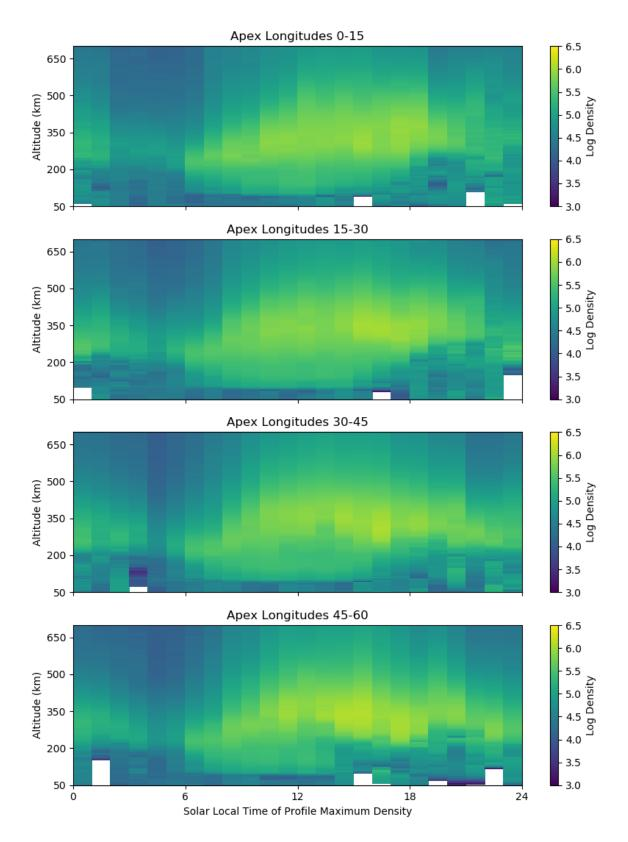
There is a gradient in the altitude distribution over longitude near sunset. Between 0-15 longitude an upward slope is seen in bottom-side density levels with local time though higher altitudes have a flatter gradient. This is consistent with the upward ion drifts reported by IVM. Between 45-60 the bottom-side ionosphere is flat with local time, while
